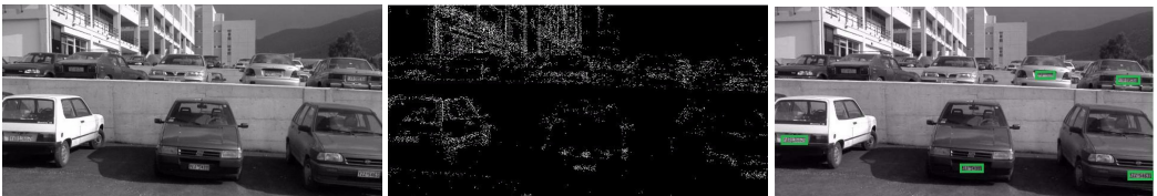
(a) Input image frame [25] (b) Background subtraction output (c) Localized objects from image b
