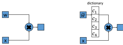
Figure 7: Multiplication with raw weights (left) and encoded weights (right).
