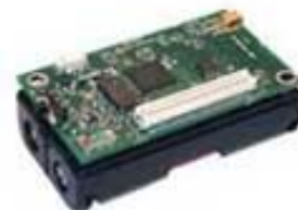
Fig. 1. Picture of a MICA2 mote. The MICA2 mote contains: (1) An Atmel ATmega128L low-power microcontroller, (2) A multi-Channel Radio Transceiver supporting 433, 868/916, or 310 MHz, and (3) A 51-pin expansion connector supports Analog Inputs, Digital I/O, I2C, SPI, and UART interfaces. The mote can have a variety of sensor types including light, temperature, and humidity sensors [13].
