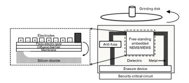
Fig. 5. Side-view of an IC using NEMS/MEMS-based devices to detect mechanical attacks. The inset shows the structure of a NEMS/MEMS cantilever.
