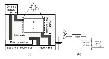
Fig. 2. (a) Side-view of an IC using photodetectors to detect optical attacks [4]. (b) Equivalent circuit diagram.
