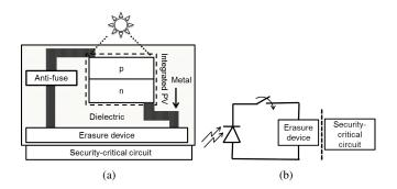
Fig. 3. (a) Side-view of an IC using energy-harvesting PV cells to detect optical attacks [4]. (b) Equivalent circuit diagram.
