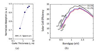
Fig. 4. (a) Calculated normalized absorption in GaAs as a function of thickness, illustrating its strong absorption properties. (b) Theoretical calculation of the conversion efficiency as a function of the absorber bandgap [22], illustrating the decline in efficiency as the bandgap is reduced.
