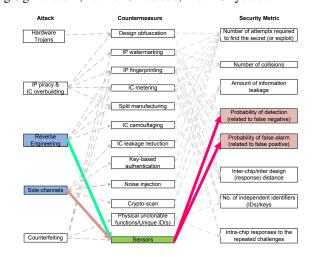
Fig. 1. Five classes of hardware attacks in [2] (left column), suggested countermeasures (middle column) and evaluation metrics (right column.) In this work, we discuss the hardware attacks, countermeasures, and metrics that are shown as colored (shaded) blocks and solid edges in the context of SHIELD.
